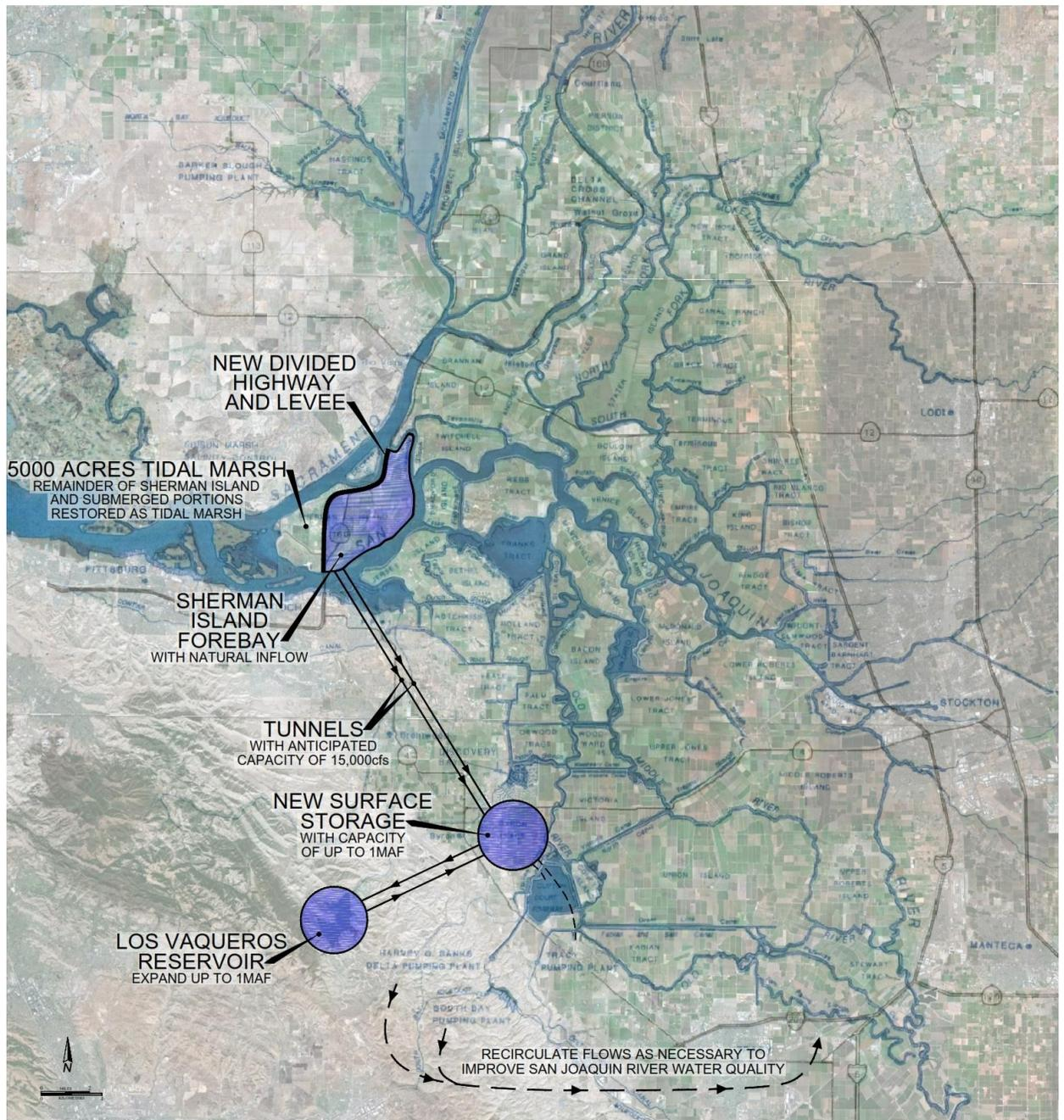
**Figure 3 – The Western Delta Intakes Concept**
